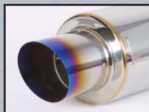
Angle cut Titanium Tip Part No.: 1058T Inlet Dia.: 3"
